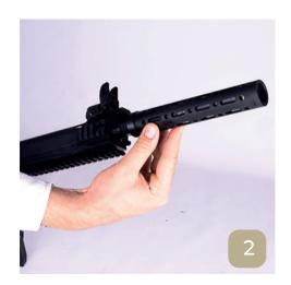
2.Muzzle break by using your hand to direction of clockwise until theread on barrel allows to disassemble muzzle completely
