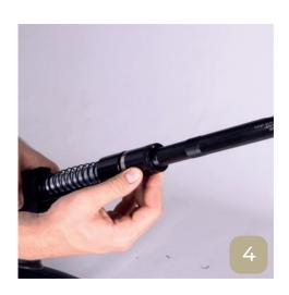
**4.**After you remove the Forearm, push "Cartridge Ramp Lock Button" and remove "Fixing Nut Barrel"
