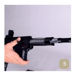
5. Remove the barrel to the rear slightly.
