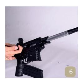
6.Pull the action bar until charging handle and the hole (charging handle lock hole) is parallel for unlocking the charging handle of Then pull the charginghandle to right side of the gun for disassembling charging handle.
