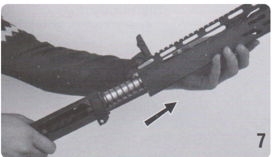
7. Remove the operating Handle, by taking it out from the front side. (Operating Handle is operational by both side Left & Right).
